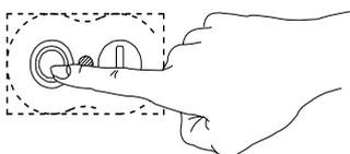
After 5 seconds the COOKING TEMPERATURE stops flashing to indicate that it has been SET.
