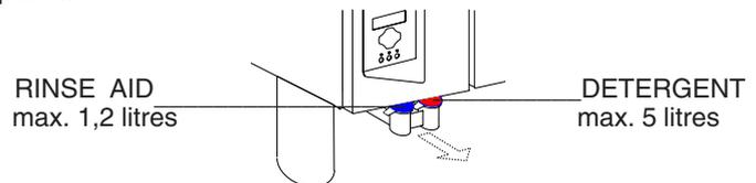
For models 20GN1/1-2/1 connect the tubes (supplied) on the left side of the oven (RH connection RED symbol for DETERGENT; LH connection BLUE symbol for RINSE AID) and insert the other ends in their respective containers (not supplied) filled with DETERGENT and RINSE AID.
